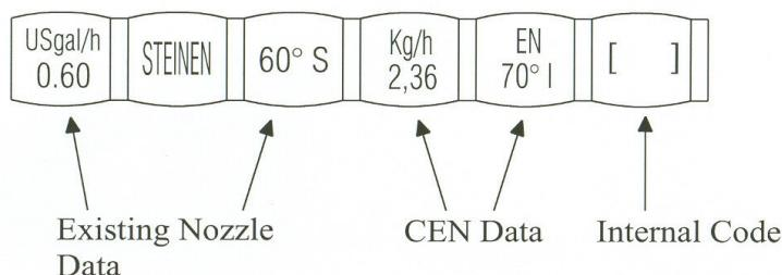
To meet the requirements and definitions of the CEN standard, dimensions, capacity (in Kg/h) and spray pattern/spray angle of each nozzle must be carefully and consistently designed and tested to meet stringent European CEN standards. Each nozzle is stamped with required CEN data to assure you this is the best performing nozzle on the market today. The performance of Steinen oil burner nozzles remains unchanged as far as capacity, atomizing angle and spray pattern are concerned.
